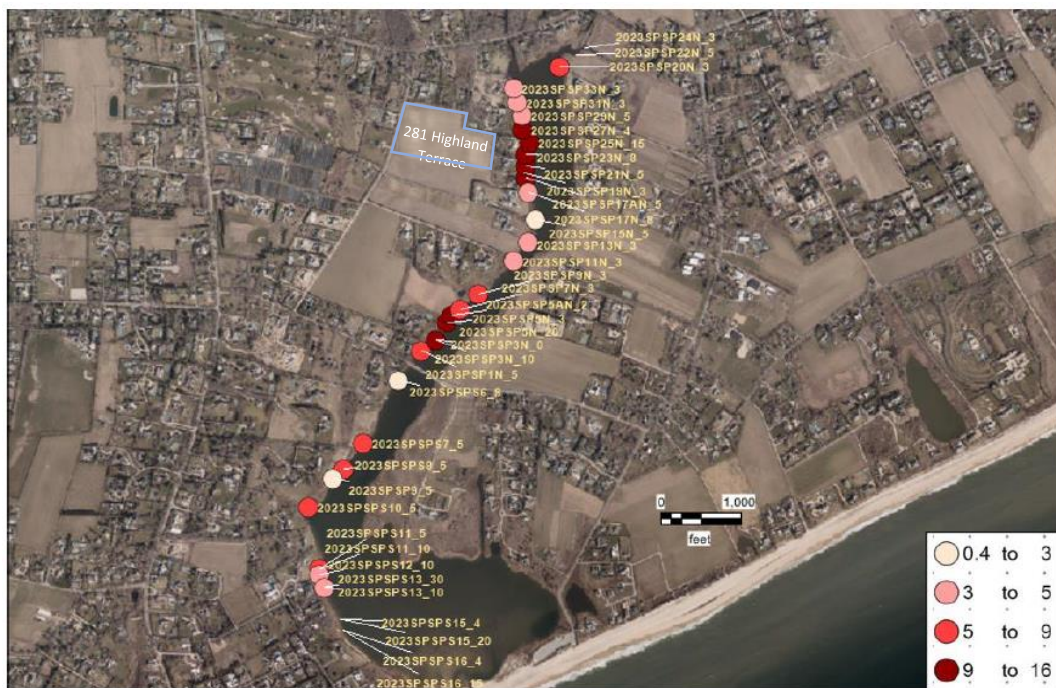
Figure 2: Porewater data collected by Coastline Evaluation Inc. in 2023 along the Sagg Pond western shoreline. Porewater nitrate values ranged from below detection ( <0.4 ) up to 16 mg N- \text{NO}_3^- /L. Sample names are in yellow. Darker red colors indicate higher nitrate concentration. 281 Highland Terrace property for proposed PRB is highlighted in blue.
