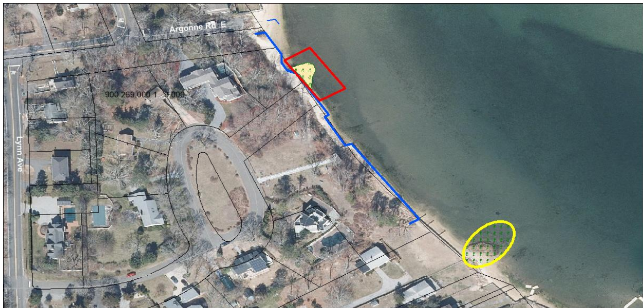
Figure 6: Aerial schematic of the proposed general location of the softened shoreline and habitat enhancement (red box) north of the existing bulkhead PRB. There is currently wooden bulkhead along the northern part of the shoreline maintained by the Hampton Hills Association. Yellow circle represents an area south of the Hampton Hills Association property where there is currently a thriving living shoreline.
