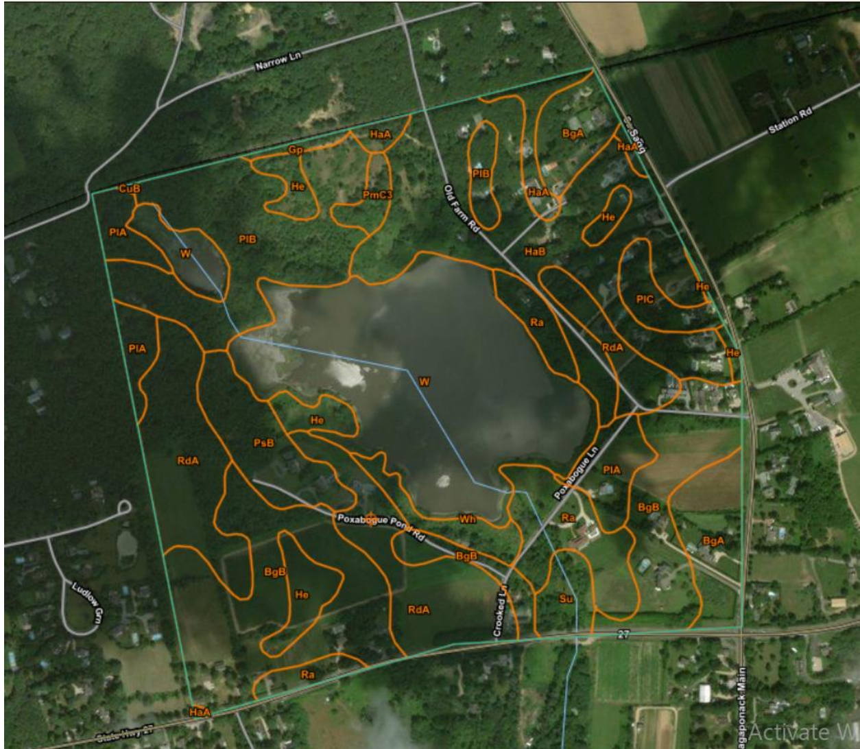
Figure B: Web-based soil survey surrounding Poxabogue Pond found at Web Soil Survey (usda.gov) . Soil in the area is dominantly Bridgehampton silt loam which consists of very deep, well drained and moderately well drained soils.
