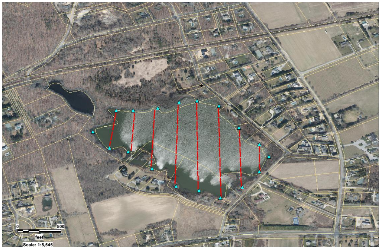
Figure 1: Map of Poxabogue Pond with porewater survey transects shown by the red dotted lines and anticipated shoreline stations for porewater and groundwater seepage measurements shown by light blue triangles.
