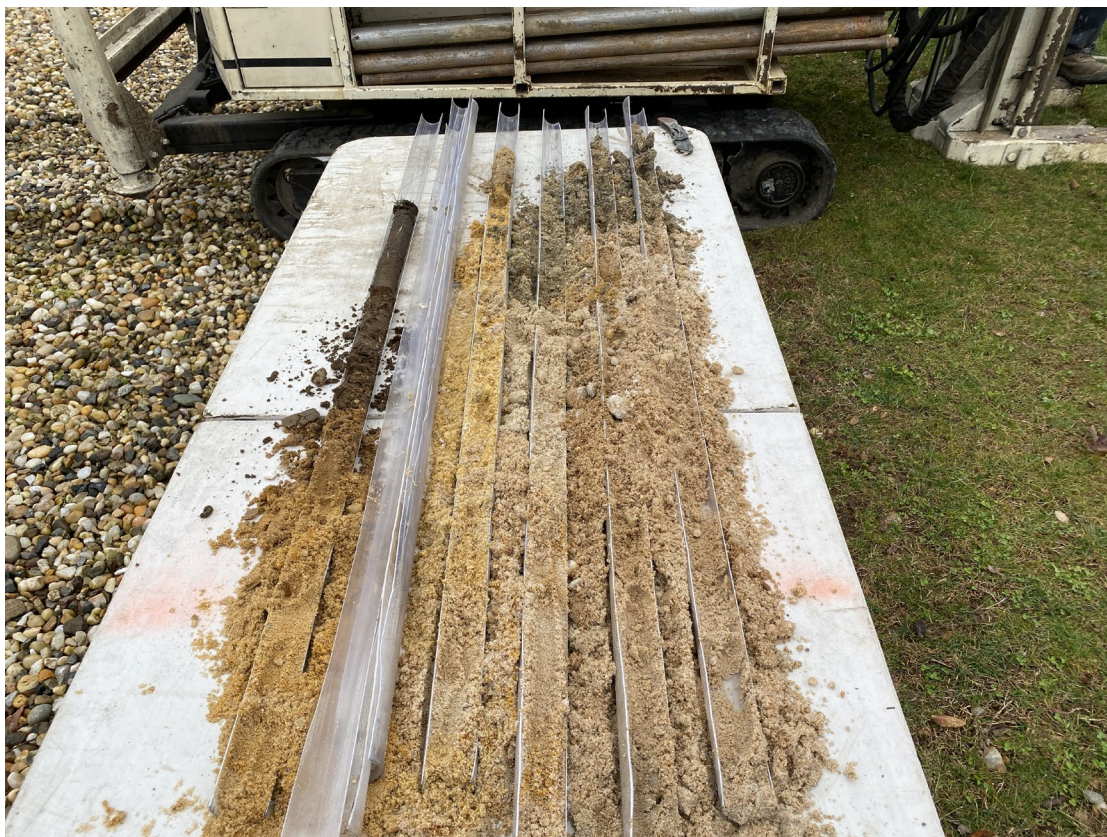
Photograph 4: Soil boring core.
