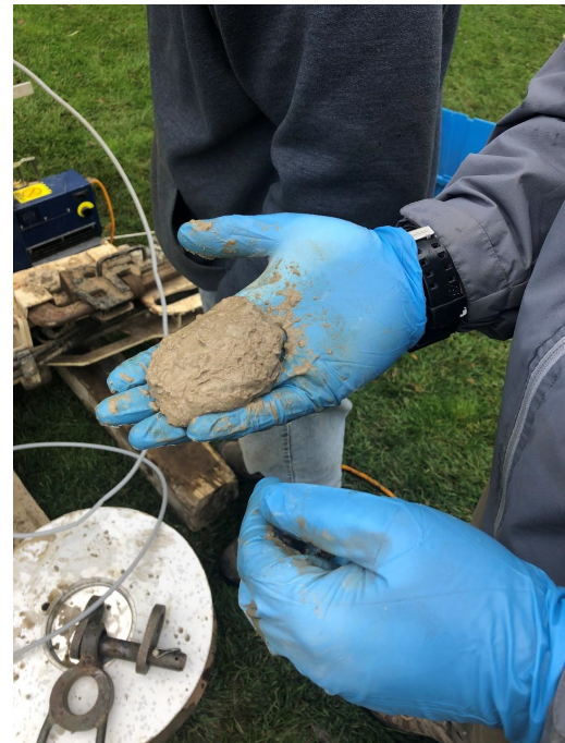
Figure 3 Sediment collected at depths beyond 120 feet below grade at LA-1 comprised of silty clay.
