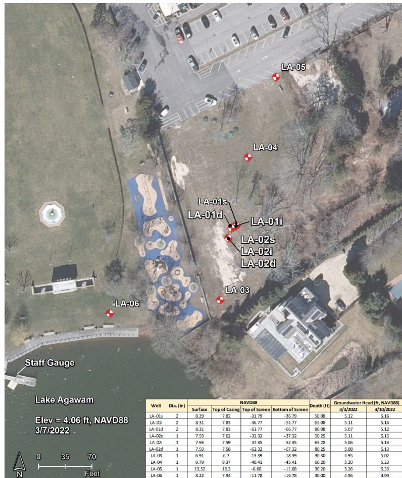
Figure 7 Monitoring wells constructed at the Lake Agawam PRB site.
