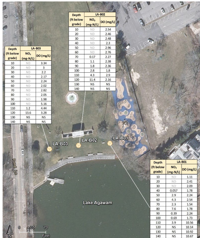
Figure 1 Nitrate and dissolved oxygen concentrations in vertical profile borings collected during Phase I.
