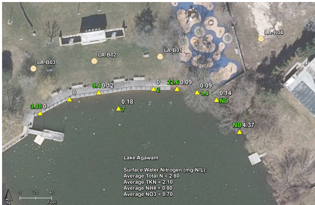
Figure 5 Nitrate (white text) and ammonium (green text) collected from porewater 1 foot below the sediment/water interface. Concentrations are in mg/L as N.
