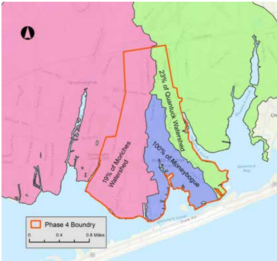
Figure 15. Extent of proposed sewer improvement area through phase 4 is outline in orange. The percent of watershed area captured by phase 4 proposal are labeled in the sections of phase 4 boundary.
