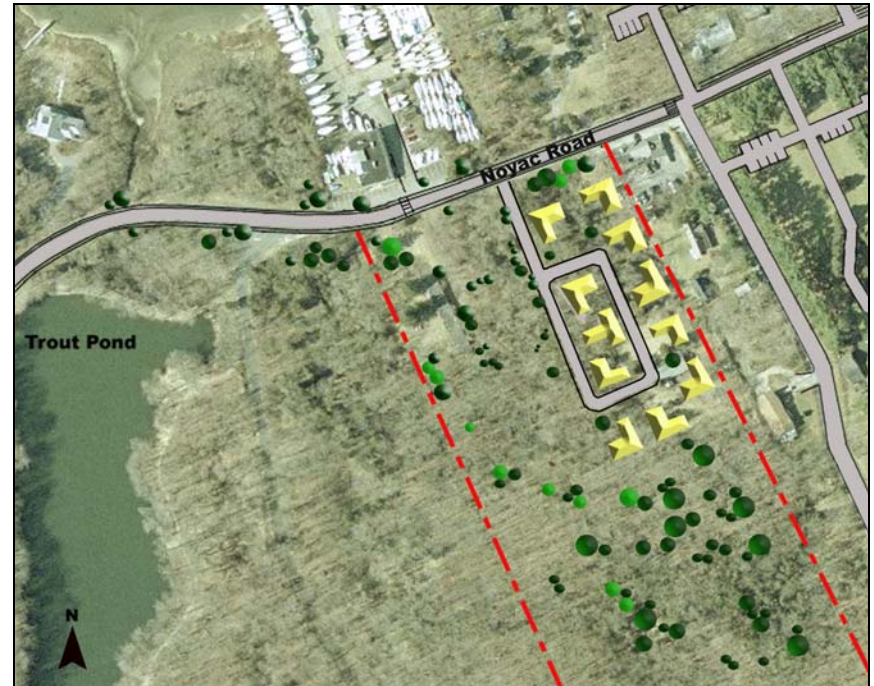
Sketch 5: Illustrative Concept – Motel Site Option 4 – Cluster housing (9 units) and 2 additional affordable housing units (total=11) in return for preservation of a minimum of 60 percent of the site as open space.
